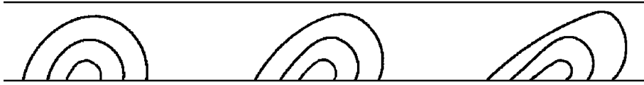
Fig. 27. Drop deformation at Re_c for the hysteresis (80^\circ, 100^\circ) (left), (60^\circ, 120^\circ) (centre) and (40^\circ, 140^\circ) (right), for the drop height h/H = 0.2, 0.4 and 0.8 .
