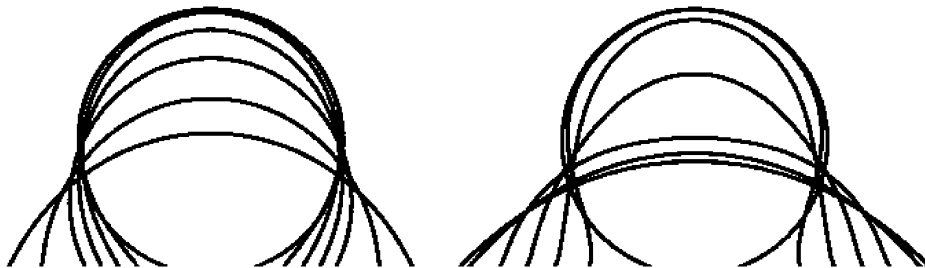
Fig. 17. Shape of the spreading drop (case LM3) at time \tau = 1.46, 2.92, 4.38, 5.84, 11.7 and 21.9 . Left: with dynamic model to describe the contact angle ( \theta = \theta_d(t) ). Right: without dynamic model ( \theta = \theta_s ).
